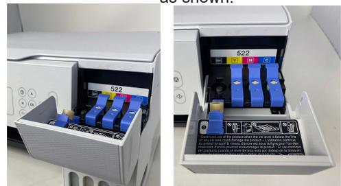
b. Position the top of the ink bottle along the slot in front of the filling port, then slowly stand the bottle up to insert it. Wait for ink to fill the tank
