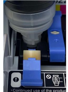
Do not squeeze the bottle. Ink flows into the tank and stop automatically when the ink tank is full.
