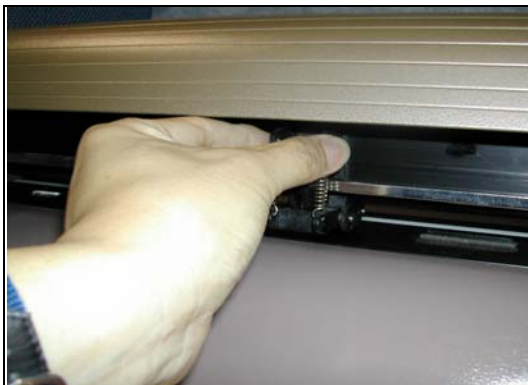
Figure 4-3 correct way to move pinch rollers
